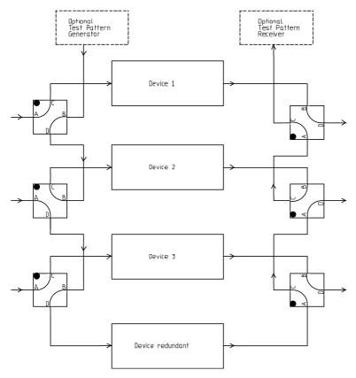
The redundant device has taken over the input and outputs of device 2. Device 2 is now connected to the optional test equipment.
